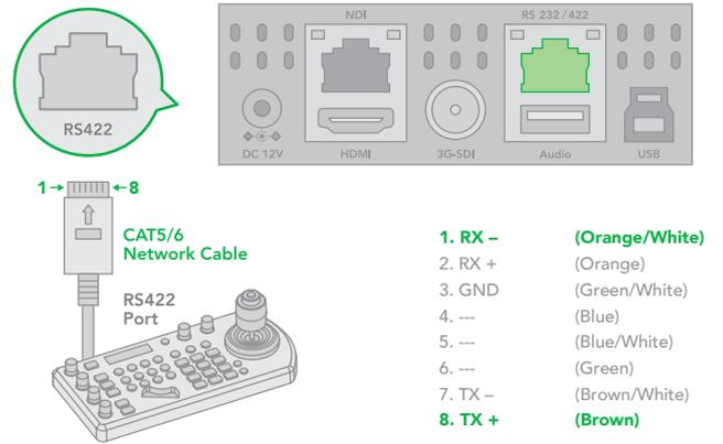
10. How to make RS422 connection and RS422 Daisy Chain multiple cameras connection with Non-Sony controller as below:
