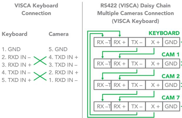
11. Use extension cables RJ45 to RS422 Phoenix connector adaptor included to make RS422 connection for your control device.
