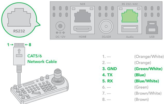
9. How to make RS232 Daisy Chain multiple camera connection with standard RS232 serial port controller as below:
